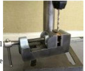
You can find them at stores that carry machine tool supplies. My feeling is that the best ones are made from steel. In particular, I like the ones with V grooves cut into the jaw plates. That lets me hold a punch straight upright or hold a rod horizontal. To find a supplier, search on "drill press vise" at sites like micromark.com, mscdirect.com/enco, smallparts.com, grizzly.com or sears.com
